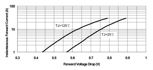
Fig.3-Typical Instantaneous Forward Voltage Characteristics
